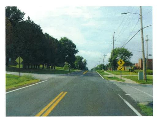
Photo 11: Pedestrian warning signs without crosswalk pavement markings crossing 155<sup>th</sup> Street at Elm Street.
